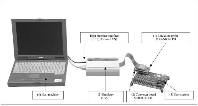
Figure 1.1 System configuration
